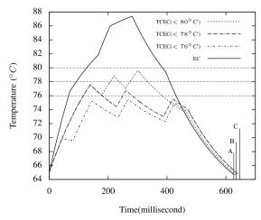
Fig. 5. EC vs TCEC. EC finishes at A.  $TCEC(<80^{\circ}C)$  finishes at B. Both  $TCEC(<78^{\circ}C)$  and  $TCEC(<76^{\circ}C)$  finish at C. The execution time of both algorithms are 0.05s and 0.07s, respectively.
