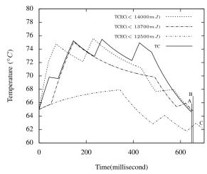
Fig. 6. TC vs TCEC. Both TC and TCEC(< 14000mJ) finish at A. TCEC(< 13700mJ) finishes at B. TCEC(< 12500mJ) finishes at C. The execution time of both algorithms are 0.04s and 0.07s, respectively.
