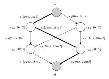
Fig. 4. JEG of TCEC. The values next to each edge are corresponding time and energy consumption.
