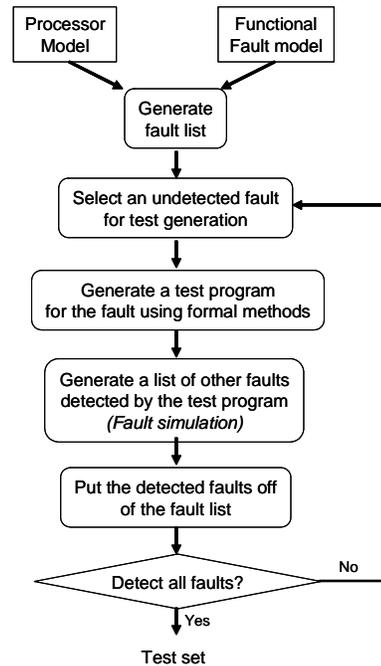
Fig. 2. Functional test generation flow
