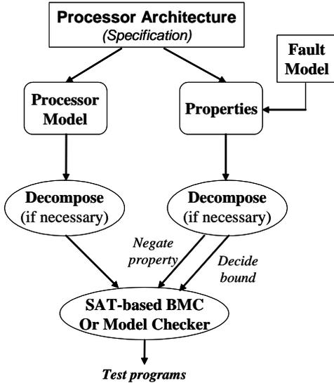
Fig. 4. Test Program Generation Methodology
