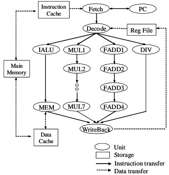
Fig. 3. Graph Model of the MIPS processor
