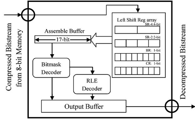
Fig. 6. Decompression engine.
