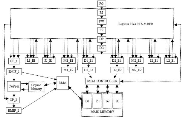
Figure 2: TI C62x Architecture with Coprocessor
