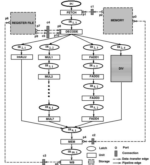
Figure 2. Graph model of simplified DLX processor
