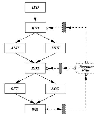
**Figure 3. An example processor with false pipeline paths**
